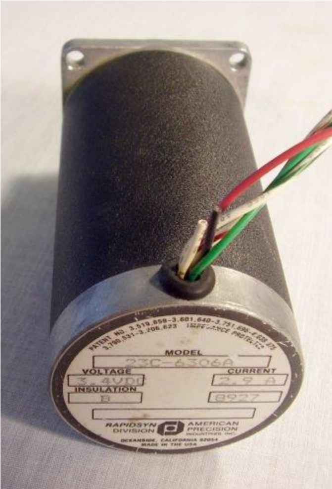
Rapidsyn stepper motor. Note coil winding's centertaps are not used.
